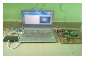
Fig. 7: Receiver Zigbee Modules is interfaced with MCU and CPLD
