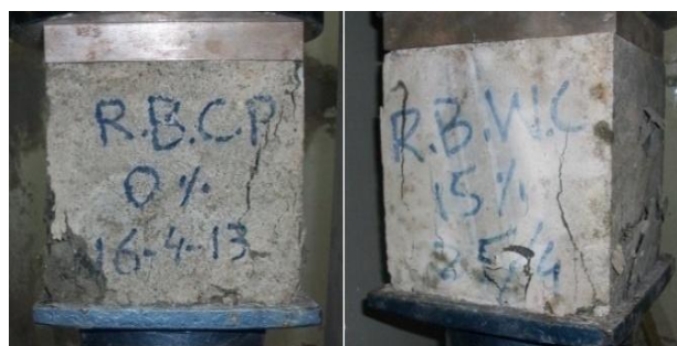
Figure 08—Samples Under Compressive Loading
