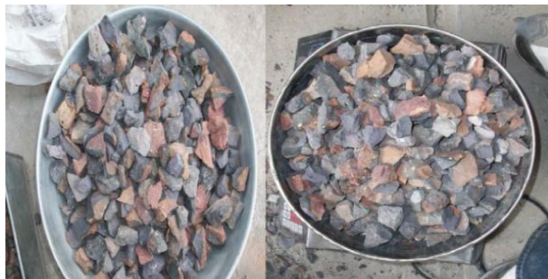
Figure 01 — Over Burnt Brick Ballast Aggregates
