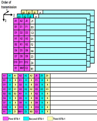
Fig. 3: Interleaving of three SONET STS-1 frame into one STS-3 frame
