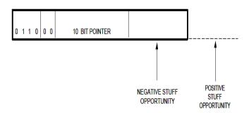
NEW DATA FLAG – INVERT 4 N BITS NEGATIVE STUFF – INVERT 5 D BITS POSITIVE STUFF – INVERT 5 I BITS
