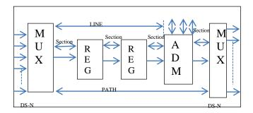
Fig. 2: SONET/SDH Architecture
