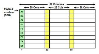
Figure 8: The Payload (SPE) of an STS-1 SONET frame
