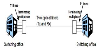
Figure 1: Early use of optical communications to replace DS-1 links betweenswitching offices. The terminating multiplexers will be inside theswitching offices. This point-to-point link is subject to failure – ringswere eventually used to provide backup.
