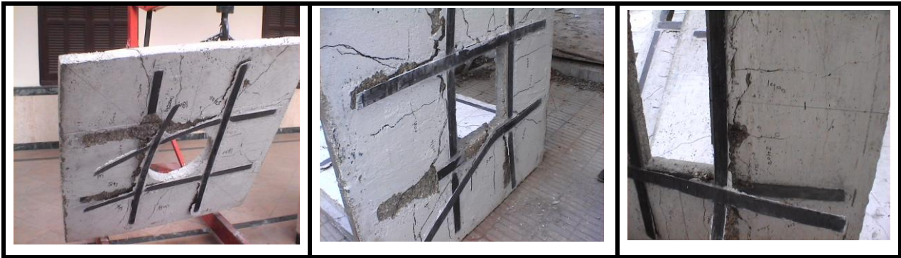
Figure 6 Failure of epoxy bonding: pull off the concrete cover
