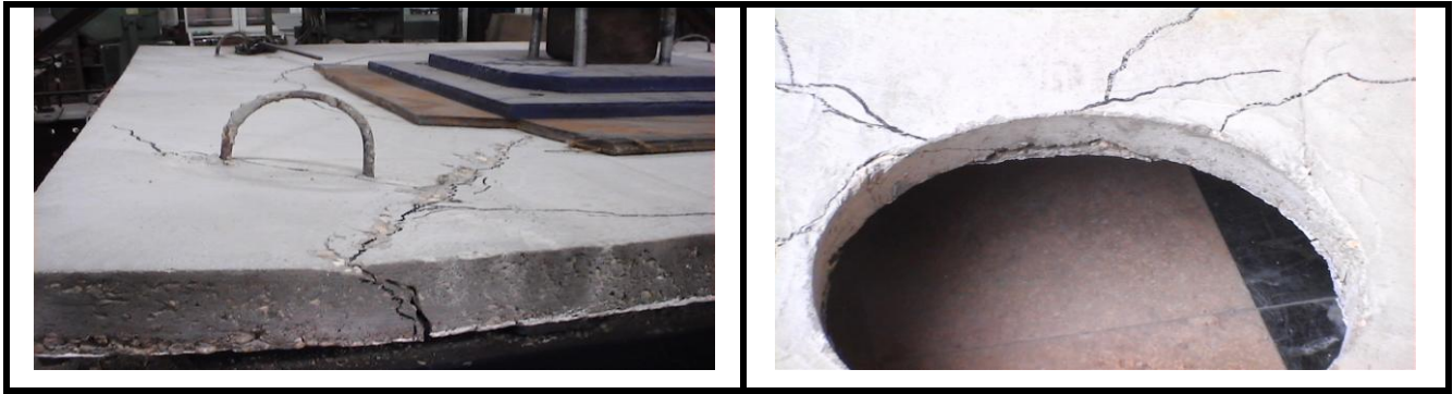
Figure 5 - Shear crack in RM and S_tMC_eCO
