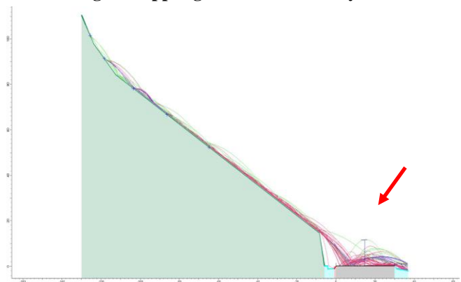
Fig. 9. Rockfall trajectories over the road break the road lamp of 12 m height shown by red arrow
