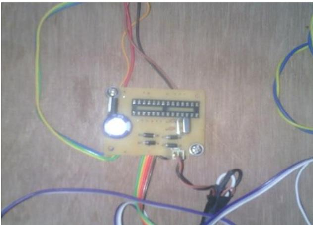
**Fig. 5: Circuit containing micro-controller IC PIC16F73, bridge rectifier and a capacitive filter.**
