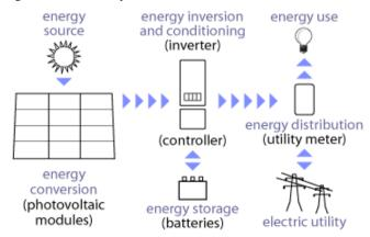
Fig. 1 Different components of PV system [3]
