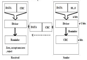
Fig. CRC sender & Receiver
