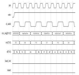
Fig. 7: Example CRC-32 Waveform From the Beginning of the Frame
