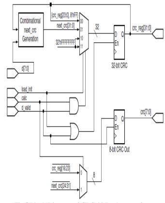
Fig.5 Block Diagram of CRC-32 Implementation
