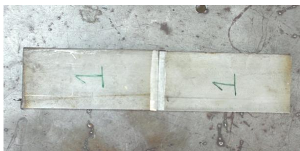
Fig 3 (a): Sample of SS202 showing V-notch before welding
