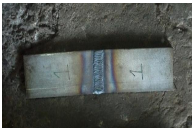
Fig 3 (b): Welded sample after TIG welding
