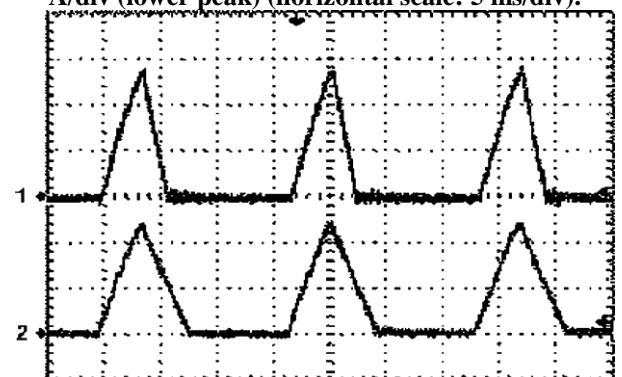
Fig. 13. Experimental waveforms: inductor L current (upper trace) and inductor L21 current (bottom trace) over several switching periods (vertical scale: 2 A/div, horizontal scale: 5 \mu\text{s} /div).
