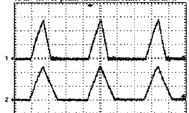
Fig. 13. Experimental waveforms: inductor L current (upper trace) and inductor L21 current (bottom trace) over several switching periods (vertical scale: 2 A/div, horizontal scale: 5 μs/div).
