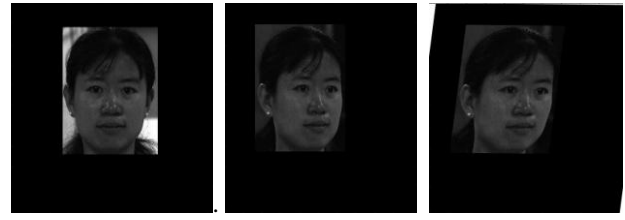
Fig.2. Image registration using the affine transformation model. Frontal and profile images are first placed at the center of a 512x512 image space.(a)Input frontal image. (b)Input profile image. (c)Profile image registered with respect to the frontal image.
