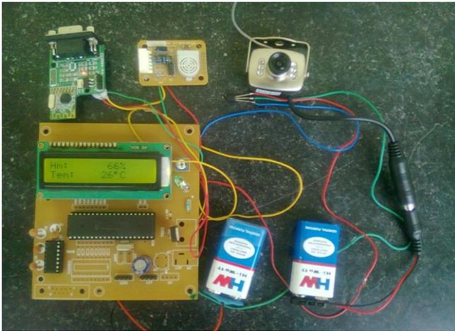
Fig. 4: Output at Normal Humidity and Temperature
