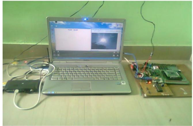
Fig. 7: Receiver Zigbee Modules is interfaced with MCU and CPLD
