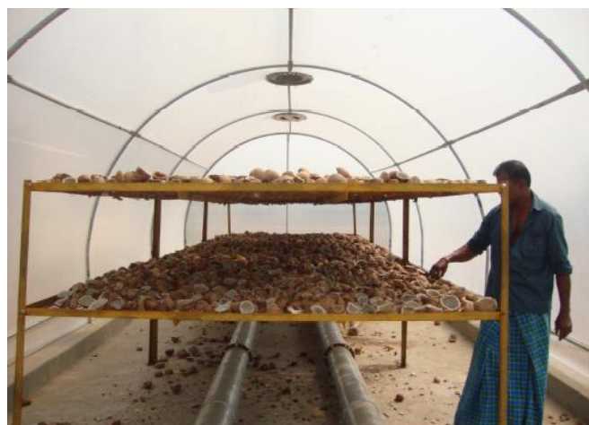
Fig. 10 Drying of Coconuts in a Solar Tunnel Greenhouse Dryer Coupled with Biomass Heater
