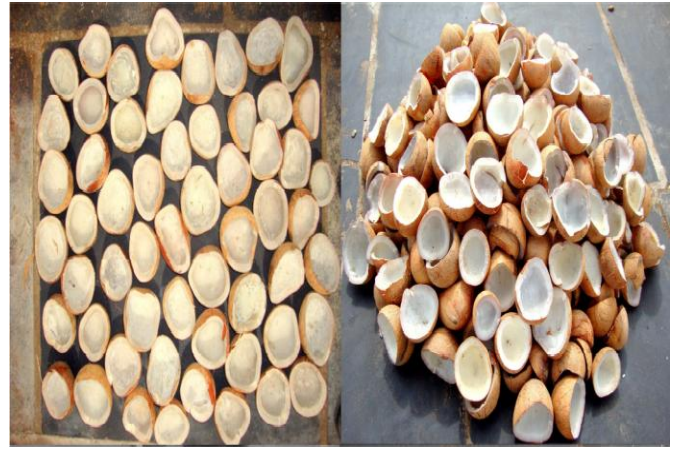
Fig. 12 Comparison of Coconuts Dried in Solar Tunnel Dryer without Biomass Heater and with Biomass Heater
