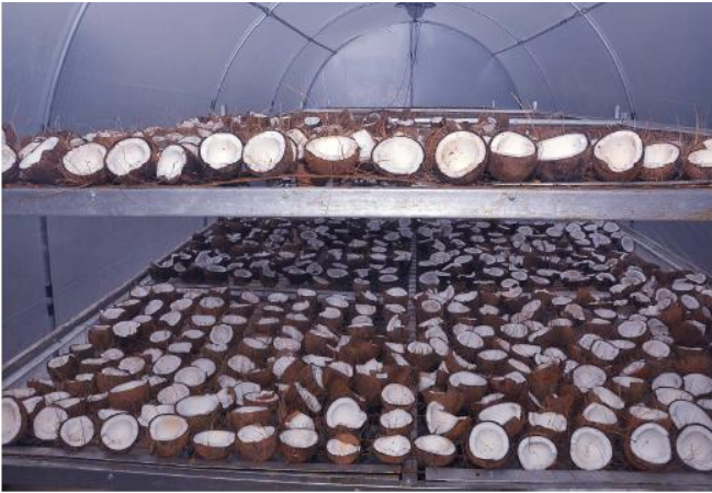
Fig. 11 Drying of Coconuts in a Solar Tunnel Dryer without Biomass Heater
