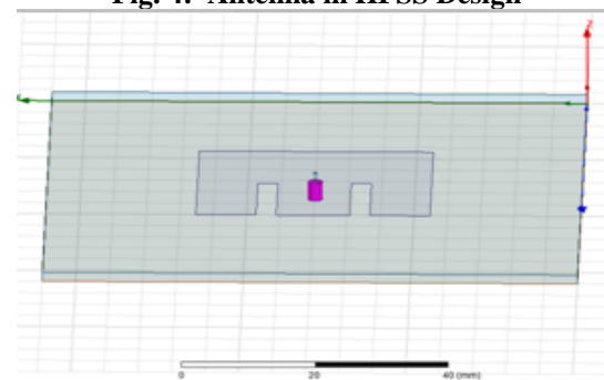
Fig. 5: Antenna in HFSS Design with probe feed
