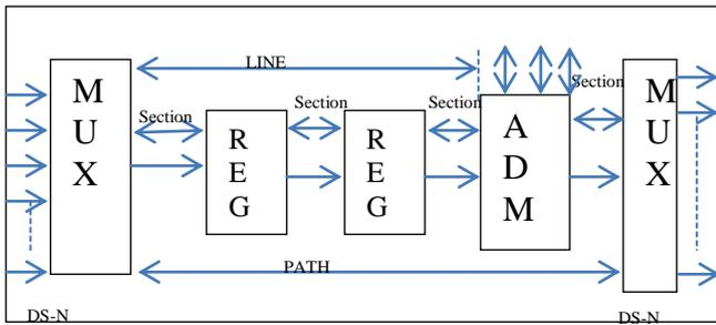
Fig. 2: SONET/SDH Architecture
