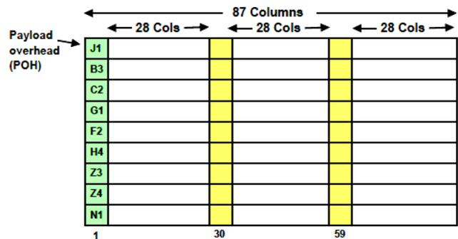
**Figure 8: The Payload (SPE) of an STS-1 SONET frame**
