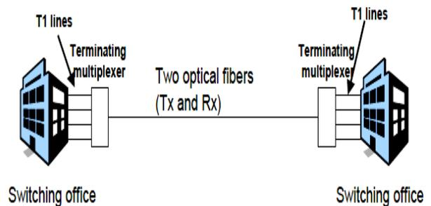
**Figure 1: Early use of optical communications to replace DS-1 links between switching offices. The terminating multiplexers will be inside the switching offices. This point-to-point link is subject to failure – rings were eventually used to provide backup.**
