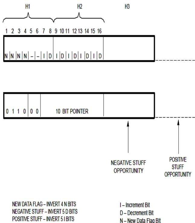
**Fig. 4: The usage of bits in the H1, H2 pointer octets.**
