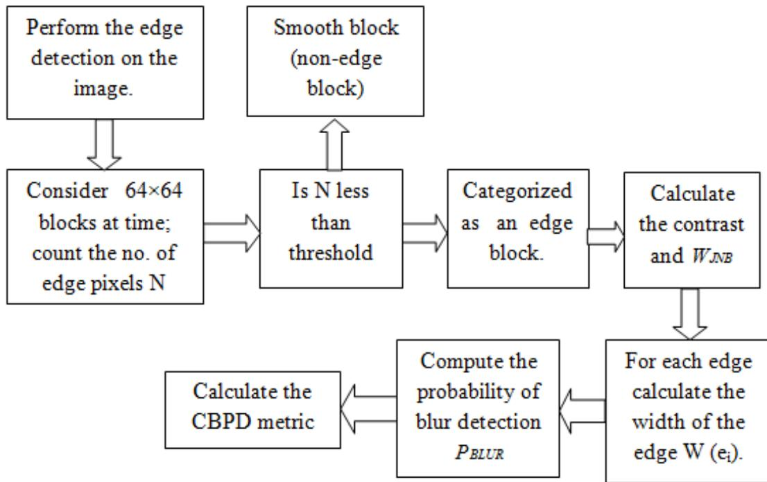
Fig. (1) Block Diagram Representing Evaluation of CPBD Metric.
