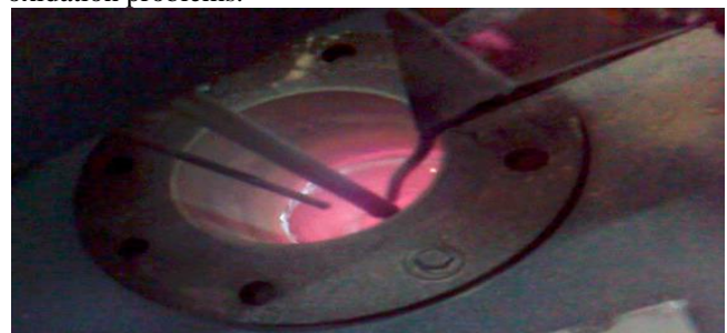
Fig .1. Stir Casting setup
