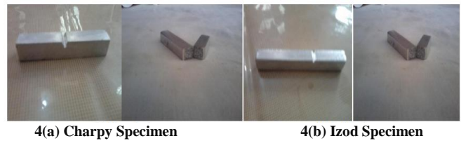
Fig4. 4(a) Izod And 4(b) Charpy Test Specimen Before and After Testing
