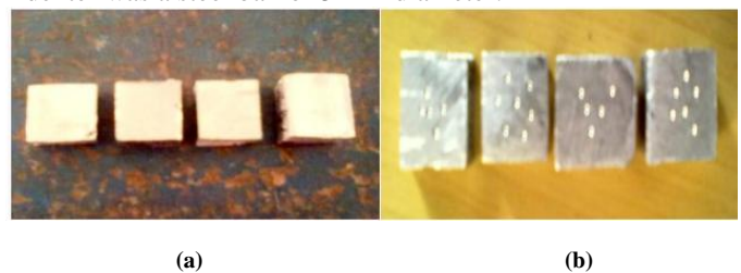
Fig 5. Hardness Test Specimen 5(a) Before and 5(b) After Testing
