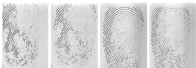
Fig. 5. An example of “failure to enroll” for fingerprints (with respect to a given fingerprint recognition system): four different impressions of a subject’s finger exhibiting poor quality ridges due to extreme finger dryness. A given fingerprint system (using a certain sensor and matching algorithm) might not be able to enroll this
