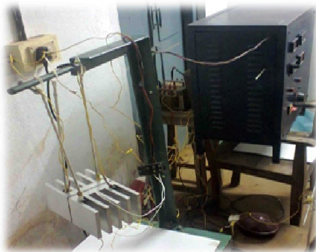
Fig.03 Photograph Heat Sink model-2 with S/H =0.25 in open air with fins in Vertical Orientation
