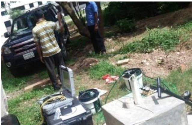
Figure 1: Installation of PS Logging Equipment (Downhole seismic method) in field (Date of testing, 02/08/13)
