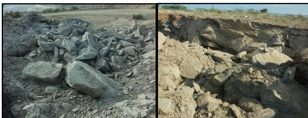
Figure 6. Rock breakage with the application of SPARSH and the face condition
