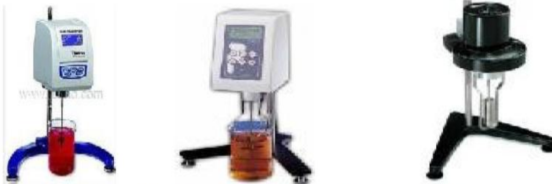
(A) Haake Viscotester VT6L/R (B) Rotational viscometer VISCO BASIC (C) Analog model of viscometer Brookfield BDRV
