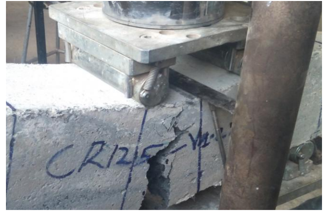
Fig. 3. Four-point bending load test and Failure mode of RTSFRC
