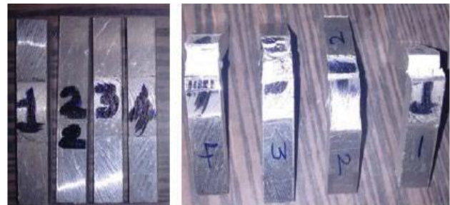
Fig. 5: Charpy's specimens of single pass before and after impact test
