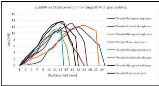
Fig. 20: Comparison between load & displacement on single & multi pass FSW
