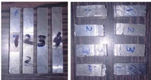
Fig. 3: Izod specimens of Multi pass before & after impact test
