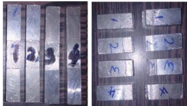
Fig. 6: Charpy's specimens of single pass before impact test and after impact test
