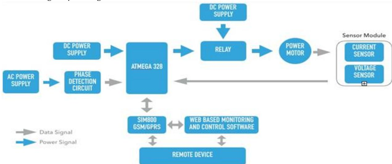
Figure 1 Block Diagram of proposed Model
