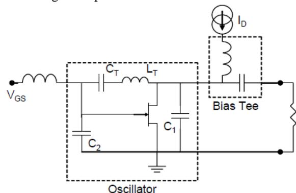
Figure.1. Design of Gouriet oscillator circuit.
