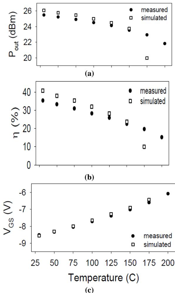
Figure.7: Analysis of oscillator parameters Pout (a), efficiency (b), and Vgs (c) respect of temperature.
