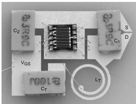
Fig.4: image of the integrated circuit passive components and transistor.
