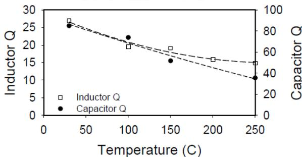
Figure.3: plotted quality of integrated circuit passive components.
