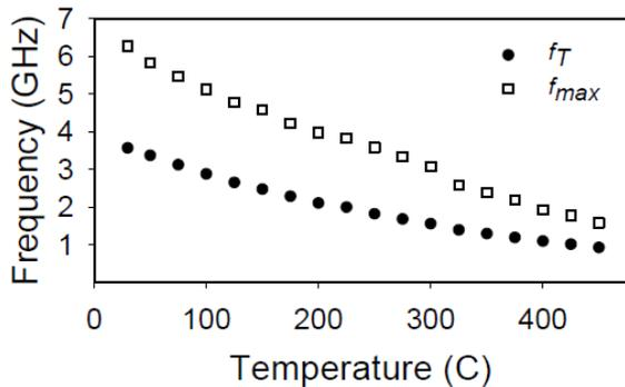
Figure.2: Transistor gain and oscillations plotted at  $I_{ds}=100mA$  &  $V_{ds}=10V$ .
