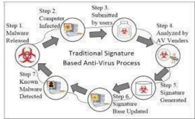
Fig.1. Steps in signature-based malware detection
