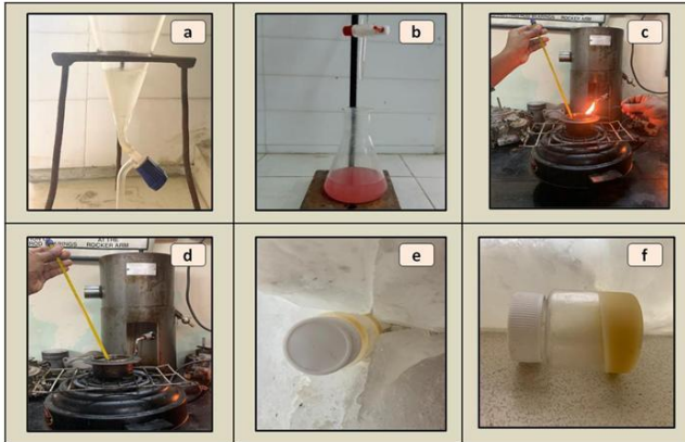
Fig. 5. Biodiesel during – (a). Methanol testing method 27/3-passed, (b). Acid value, (c). Fire point, (d). Flash point, (e). Cloud point, (f). Pour point.
